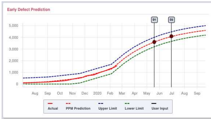
Fig. 14: Early arrival defect prediction with target values at D1 and D2, actual defect data overlaid
