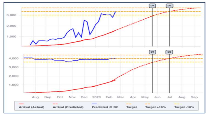
Fig. 16: Stability and accuracy of early defect prediction vs. defect trend analysis
